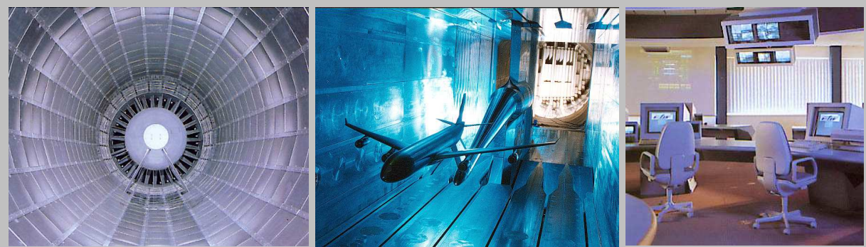
Some components of a windtunnel (f.l.t.r.): fan, downstream, operating area.
