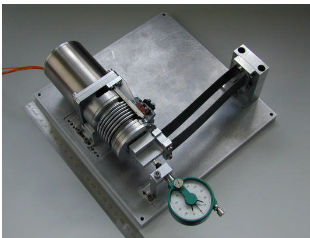
Figure 5. Test device including linear actuator without planetary gear mounted and cut through this actuator.
