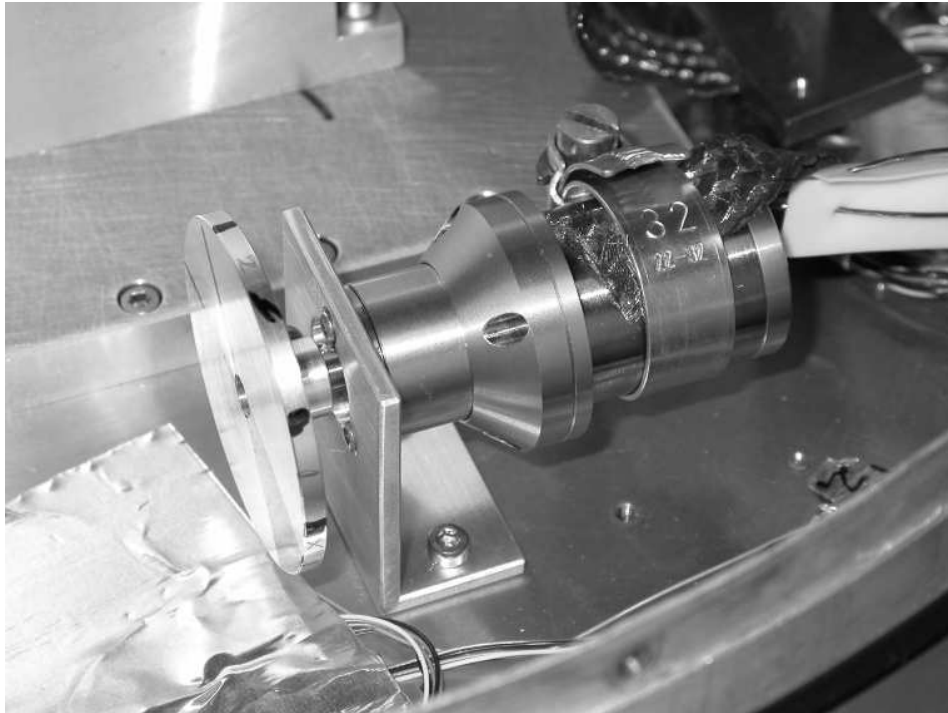
Figure 2. Rotational cryogenic actuator (stepper motor with Harmonic Drive gear) mounted in the test cryostat.
